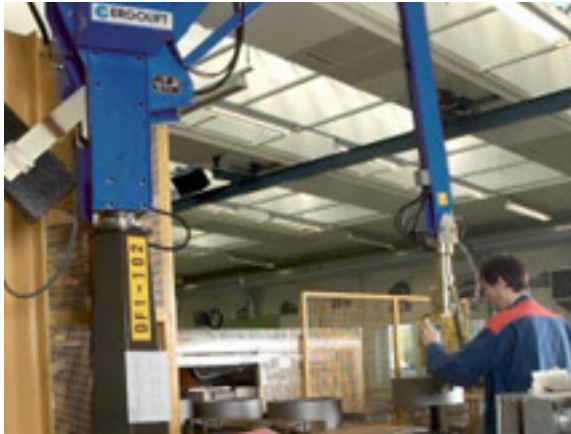
The electronic control system of the Ergobalancer automatically balances the load so that the operator can move the load conveniently and safely simply by pushing in the desired direction.
