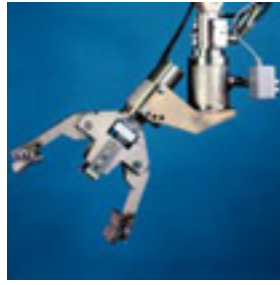
EGH20/EGH25 Vertical/sloping installation. The slope angle is adjustable in steps 0/15/30/40° about the beta axis. EGH20 With clamp mounting for stepless adjustment about the gamma axis. EGH25 Manually rotatable 340° about the gamma axis.
