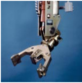
EGH55/EGH65 Powered tilting travel 90° about the beta axis. Centrally located gamma axis. EGH55 With clamp mounting for stepless adjustment about the gamma axis. EGH65 Manually rotatable through an unlimited angle about the gamma axis.
