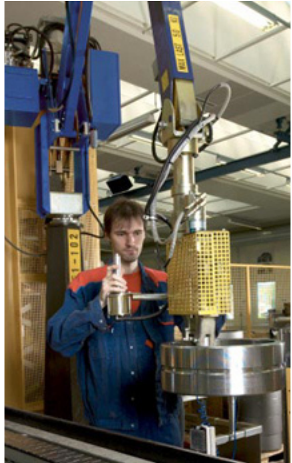
The electronic control system of the Ergobalancer automatically balances the load so that the operator can move the load conveniently and safely simply by pushing in the desired direction.
